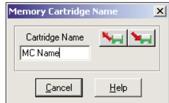
If the PC is connected to the PLC, the PLC-icon buttons will become active. When the PLC-icon buttons are active, you can also transfer the name to the PLC or transfer an existing name from the PLC into *DirectSOFT 5*. Transferring the Memory Cartridge name into the PLC transfers the name directly to the Memory Cartridge.
