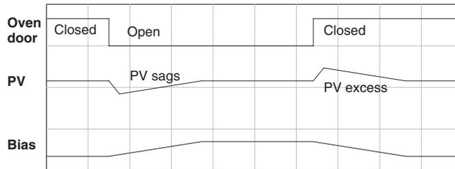
First, we record the amount of bias change the loop controller generates when the door opens or closes. Then, we write a ladder program to monitor the position of an oven door limit switch. When the door opens, our ladder program reads the current bias value from V+04, adds the desired change amount, and writes it back to V+04. When the door closes, we duplicate the procedure, but subtracting desired change amount instead. The following figure shows the results.
